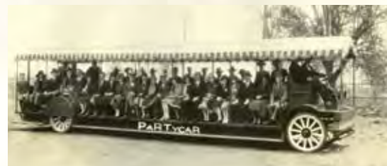
Twenty-five electrical buses, called The PaTy Car, shuttled visitors throughout the Exposition. Operated by the Philadelphia Rapid Transit Co. (PRT), each bus sat 40 people and could reach a speed of 8 MPH.
